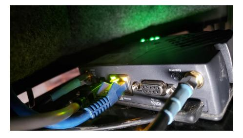
3) If the operator is experiencing the 'loss of GPS' issue when the modem is powered up, the user should unhook the 'Cell' coax antenna cable leading to the 'Diversity' port. (See Below)
